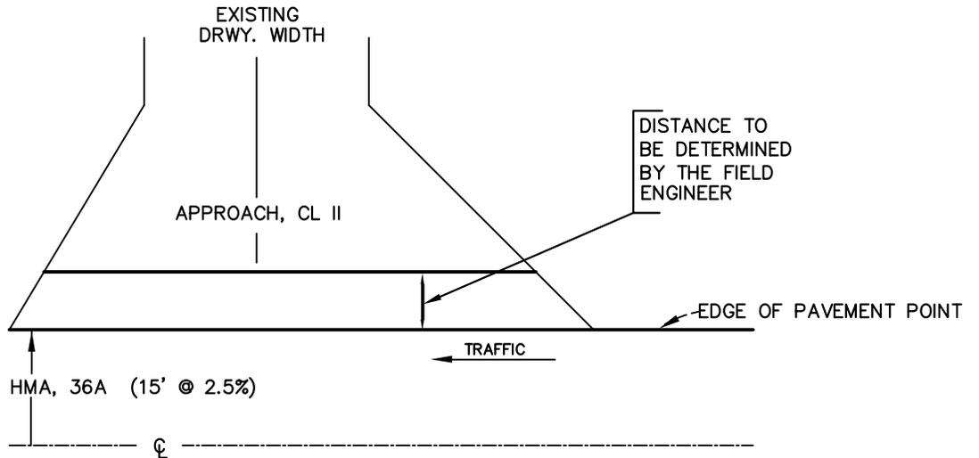
MATERIAL FOR APPROACH, CL II (23A) SHALL BE ACCEPTED AT THE PROJECT SITE WITH LOAD TICKETS LABELED "APPROACH, CL II" ONLY. APPROACH, CL II SHALL BE PLACED TO PROVIDE A SMOOTH TRANSITION FROM THE SHOULDER POINT GRADE TO EXISTING DRIVEWAY GRADE AT A DISTANCE TO BE DETERMINED BY THE ENGINEER.
